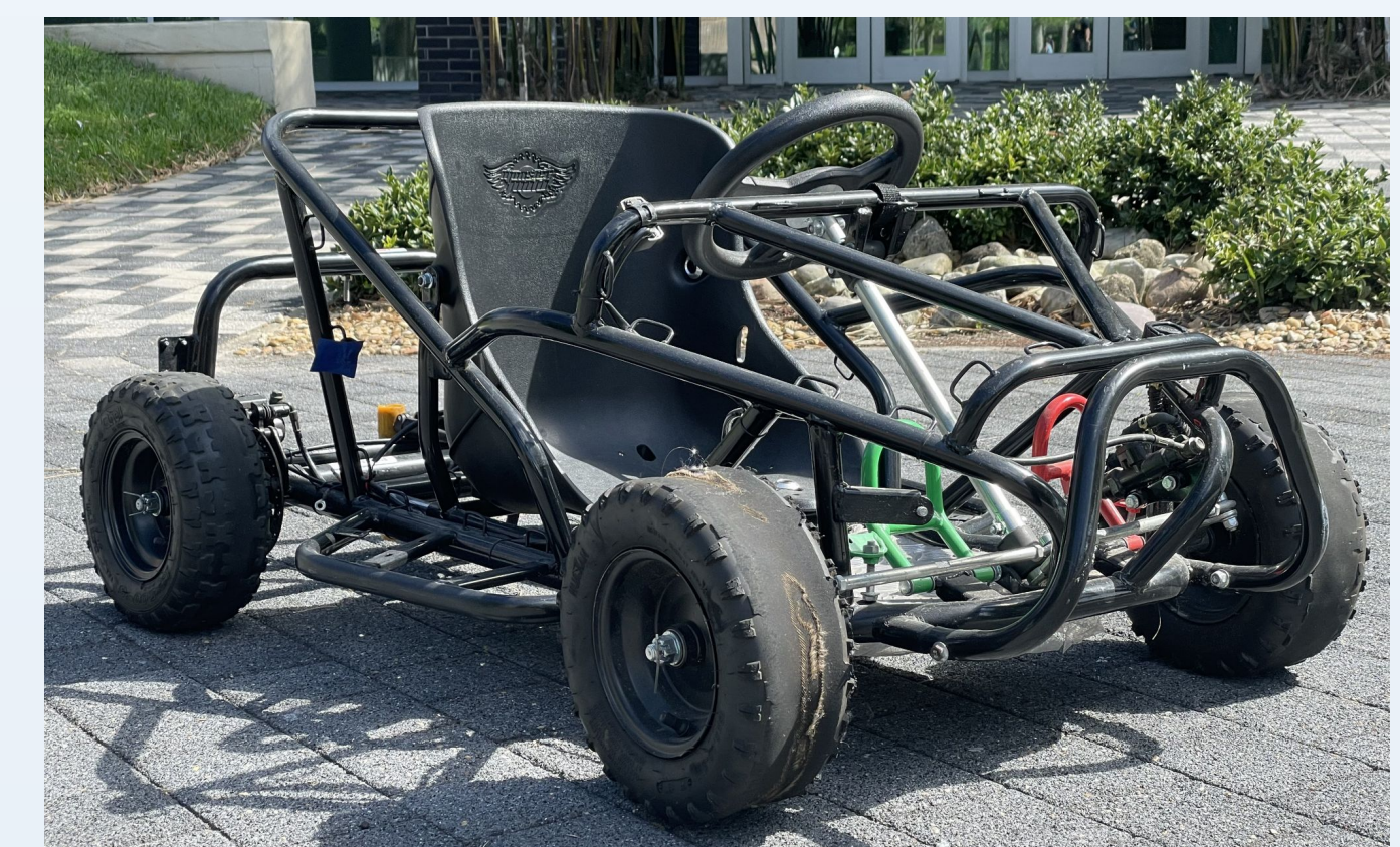
Figure 5. Super State Racer Prototype Frame
